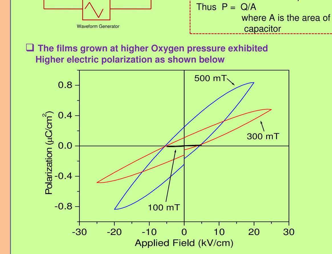
Fig. 10: Electric Polarization as a function of applied electric field for the films grown at various oxygen pressures. The polarization measurements were performed using Precision LC from Radiant Technologies
