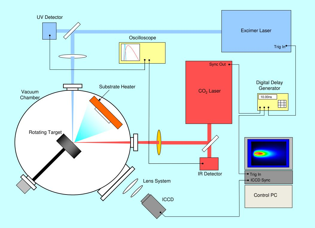
Fig.3 : The schematic diagram of the dual-laser deposition system (248 nm KrF excimer laser and 10.6  $\mu$ m CO<sub>2</sub> laser) with the ICCD imaging system (PI-MAX:512 UNIGEN)
