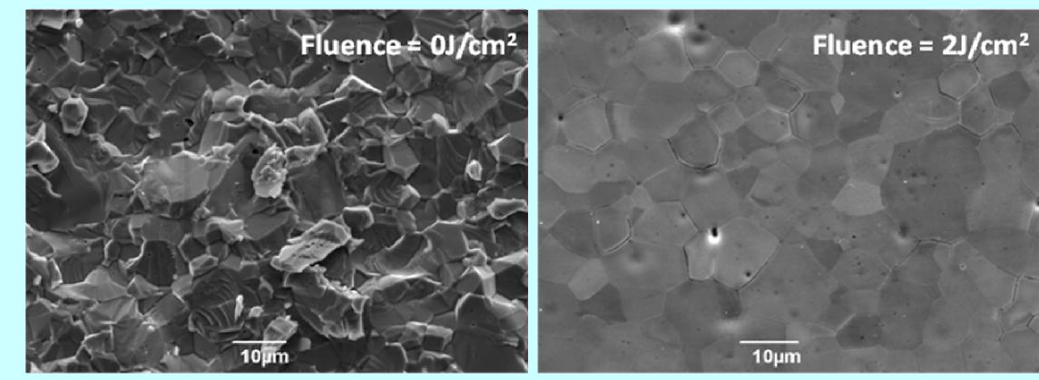
Fig.4 : SEM pictures of unablated (left) and 2J/cm<sup>2</sup> ablated (right) surface of ZnO ceramic target
