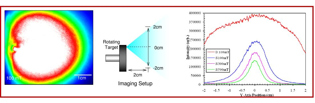
Figure 7: ICCD imaging (left), image set up (middle) and total emission intensity plot for single-laser 2 J/cm<sup>2</sup> (100 mT O<sub>2</sub>, 300mT O<sub>2</sub> and 500 mT O<sub>2</sub>) and dual laser  $(2J/cm^2 UV and 2J CO_2)$  at 100 mT O<sub>2</sub>. Intensity range is from 0 to 300000
